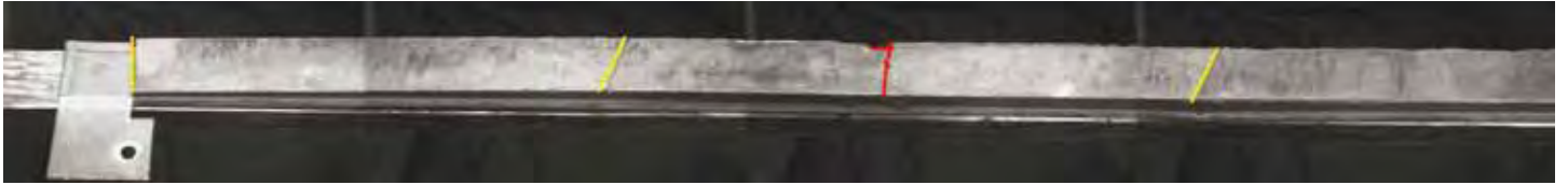
The detection of cracks on a train pantograph carbon conductor bar
