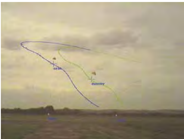
The tracking of an ejector seat and a manikin during testing
