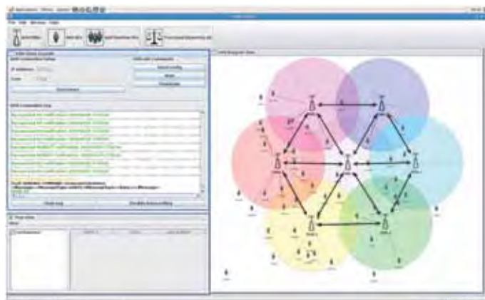
Figure 1: Automatic establishment of X2 interfaces using ANR
