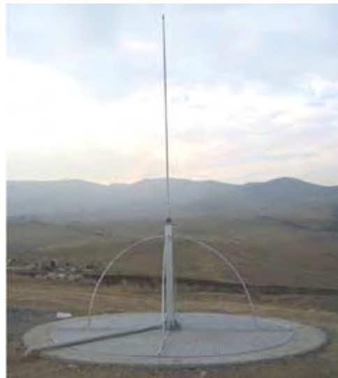
Field deployed Roke HF Crossed Loop Antenna (static location - Eurasia)
