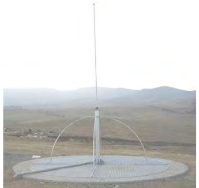
Figure 7: 1x element of Roke 8-Element HFDF Array incorporating Roke Compact Crossed-Loop (Central Europe)
