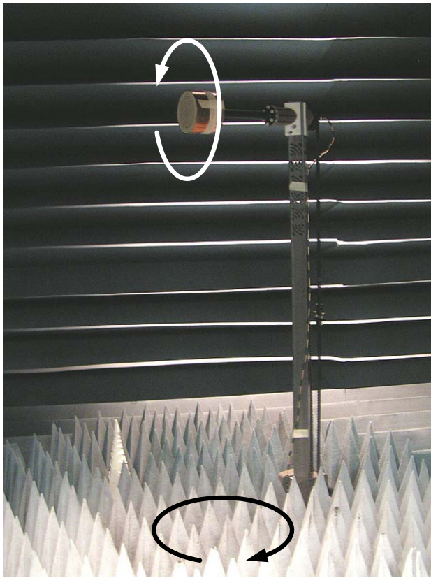
Figure 7. A view inside the anechoic chamber showing the axes of rotation
