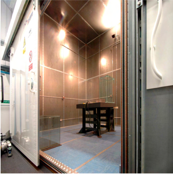
Figure 4. HVTF – High Voltage Chamber.
