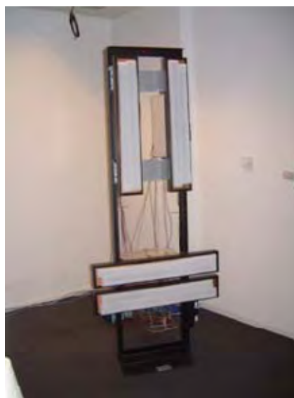
Figure 3: UWB 3D Imager demonstrator experimental set-up
