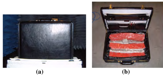
Figure 10: (a) Briefcase on polystyrene block (b) containing simulated bomb plastic and ball bearings
