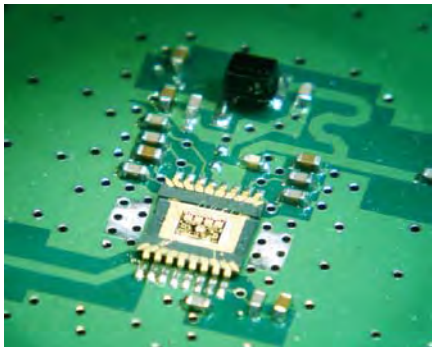
Figure 1: A plastic packaged MMIC (lid removed), with support components, on an FR4 PCB.
