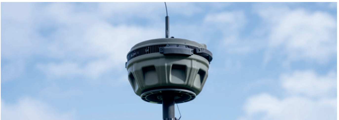
3 Roke's Perceive ( https://www.roke.co.uk/products/perceive-multi-role-mr ) can separate multiple co-channel signals and give bearings on to multiple targets.
